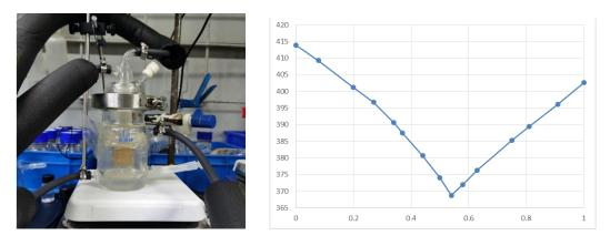
Figure 6 Melting crystallization experiment facility and phase diagrams.
