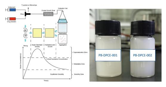
Figure 8 Nanosuspension production of two APIs using a plug flow crystallizer.
