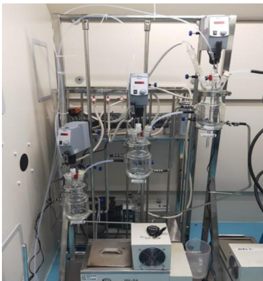
Figure 7 A three-stage MSMPR crystallizer.
